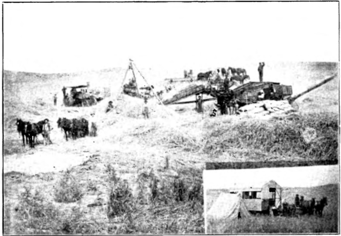
Steam Threshing Outfit of W. Moreland Threshing Three Thousand Bushels of Wheat Per Day.
